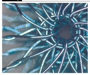
PFO occluders of competitors are made from several wires, with the need to fix the loose ends with clamps.
